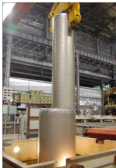
Figure 6. A 26" billet of 7050 alloy being removed from the pit.
