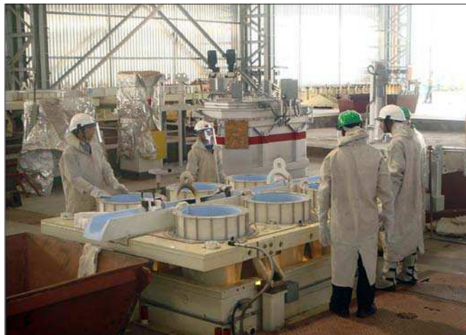
Figure 7. 650 mm diameter tooling for hard alloy casting.
